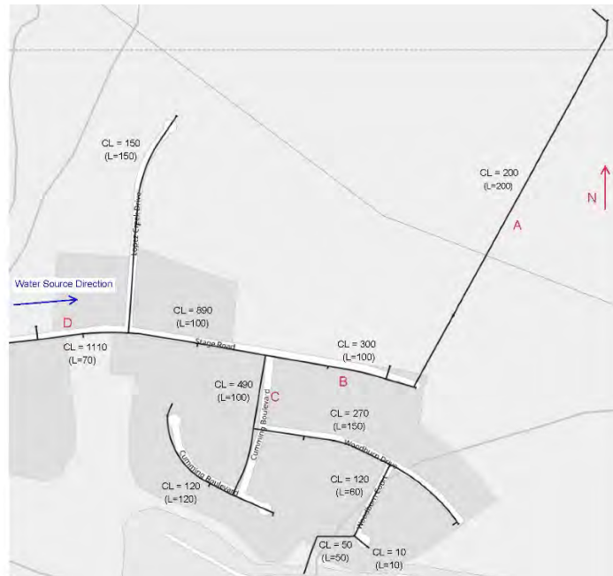
FIGURE 3-2: EXAMPLE OF DETERMINING WATER CRITICAL LENGTH
