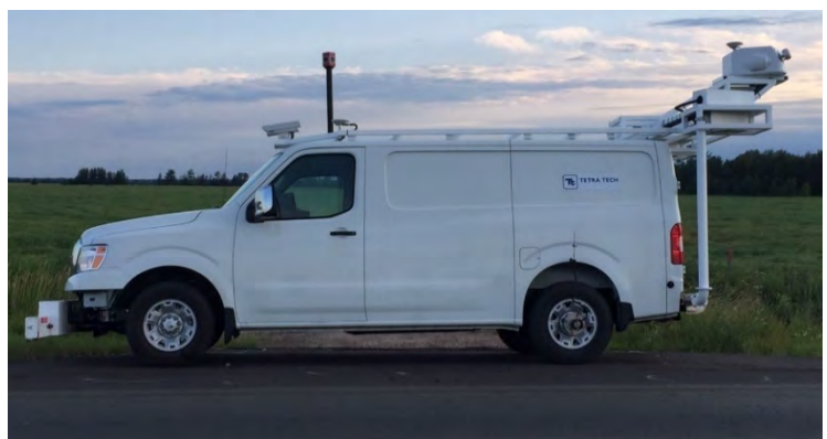
Figure 2 - Tetra Tech's PSP-7000 Vehicle
