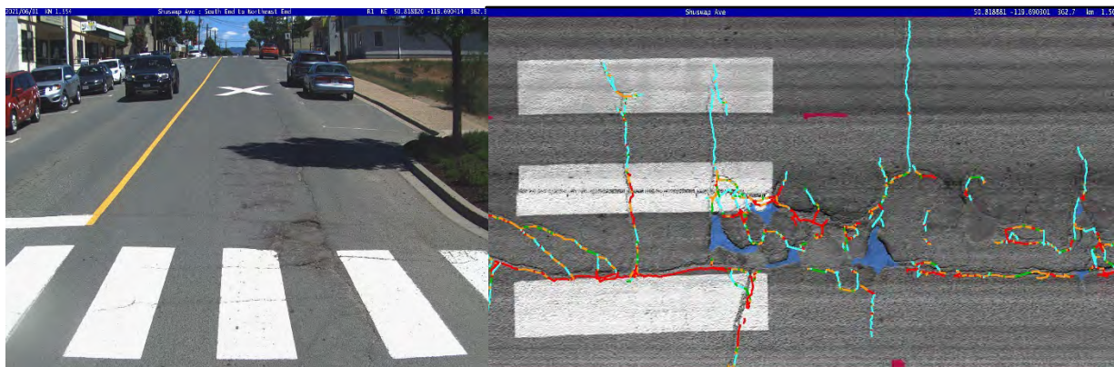
Figure 5 - Example of PSP-7000 Digital Image Log (Front & Top Down)
